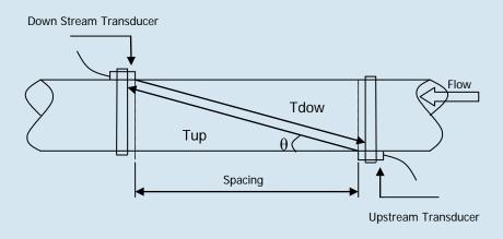
$$V = \frac{M \cdot D}{\sin 2\theta} \times \frac{\Delta T}{T_{up} \cdot T_{down}}$$
